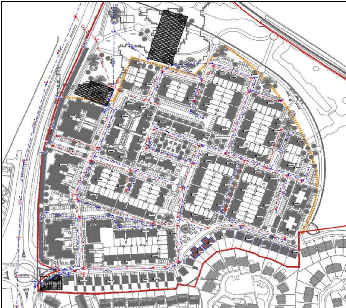
Figure 4-2 Proposed Surface Water Systems Layout (Source: HOM Civil Engineering Report)
